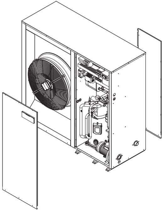
**Refrigerant circuit.** It is contained inside a compartment separated from the air flow to simplify maintenance and control operations.
