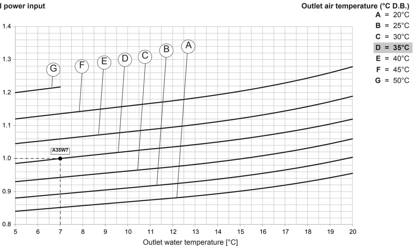
The standard performances refer to a 5°C temperature difference between the water entering and leaving the heat exchanger and to operation of the unit with all fans at nominal or maximum speed. A  $0.44 \times 10^{-4}$  m<sup>2</sup> K/W fouling factor has also been considered with the unit installed at zero meters above sea level (Pb = 1013mbar).
